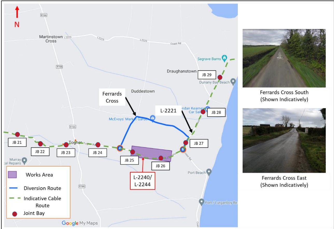
Figure 4-12: Diversion 12 - Joint Bay No. 25 to Joint Bay No. 26 (Source: Google My Maps).
