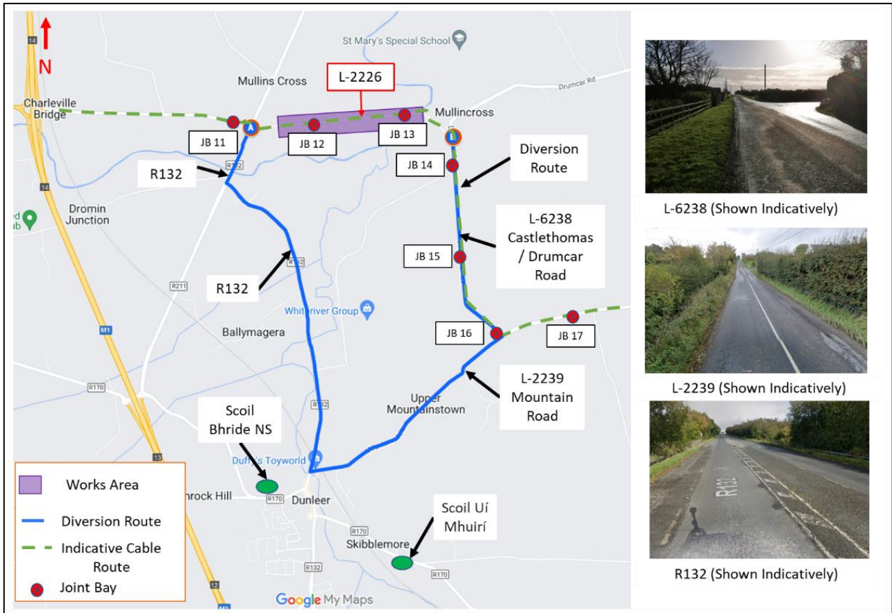
Figure 4-4: Diversion 4 - Joint Bay No. 12 to Joint Bay No. 13 (Source: Google My Maps).
