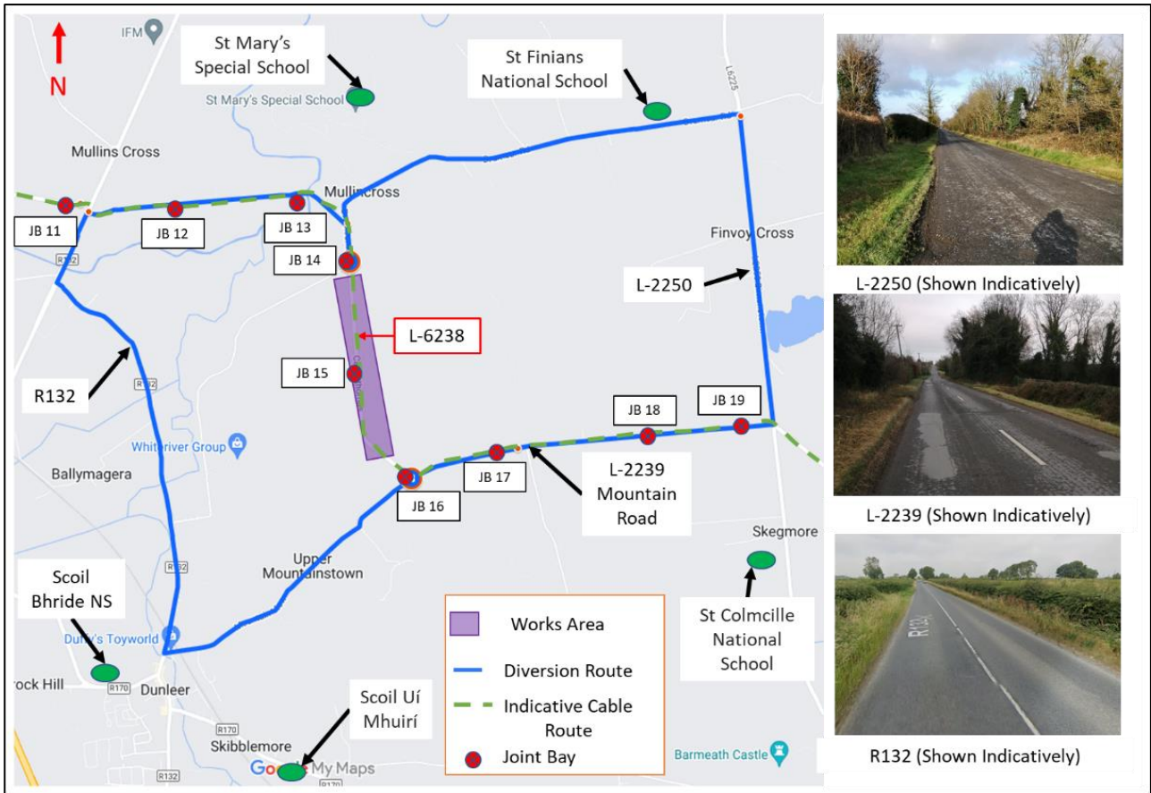
Figure 4-6: Diversion 6 - Joint Bay No. 14 to Joint Bay No. 16 (Source: Google My Maps).
